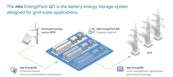
A complete plant design may consist of multiple building blocks. Each block is designed for 4.39 MVA nominal charge and discharge rating up to 17.89 MWh, consisting of up to 48 battery racks.
